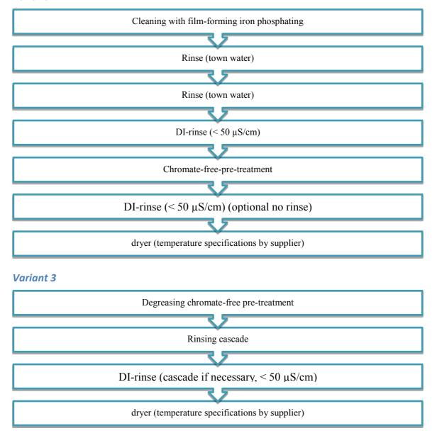
Beside the chromate-free corrosion protection process (product name) the used process variant is specified in the certificate of approval. As the approval test only includes the corrosion protection characteristics of the chromate-free pre-treatment product, the cleaning product will not be specified.
